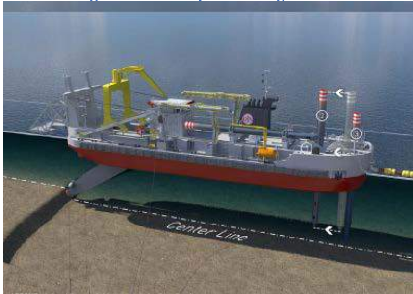
Figure E-7: CSD Spud Shifting Process
