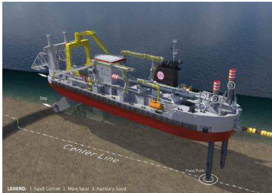
Figure E-6: CSD Stepping Process
