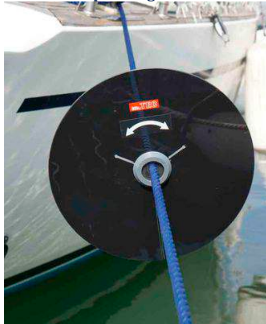
Figure 15-1: Rat-proofing collars and hawsers
