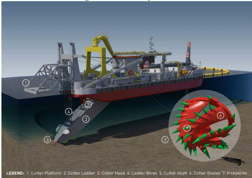
Figure E-1: General layout of a CSD
