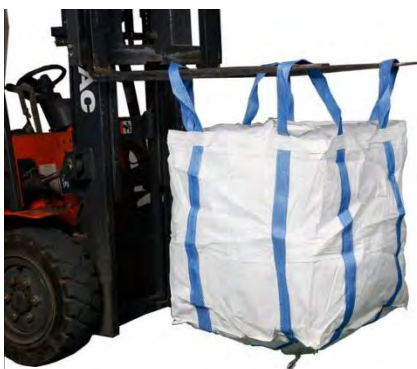
Figure 3: Bagged concrete washout removal system
