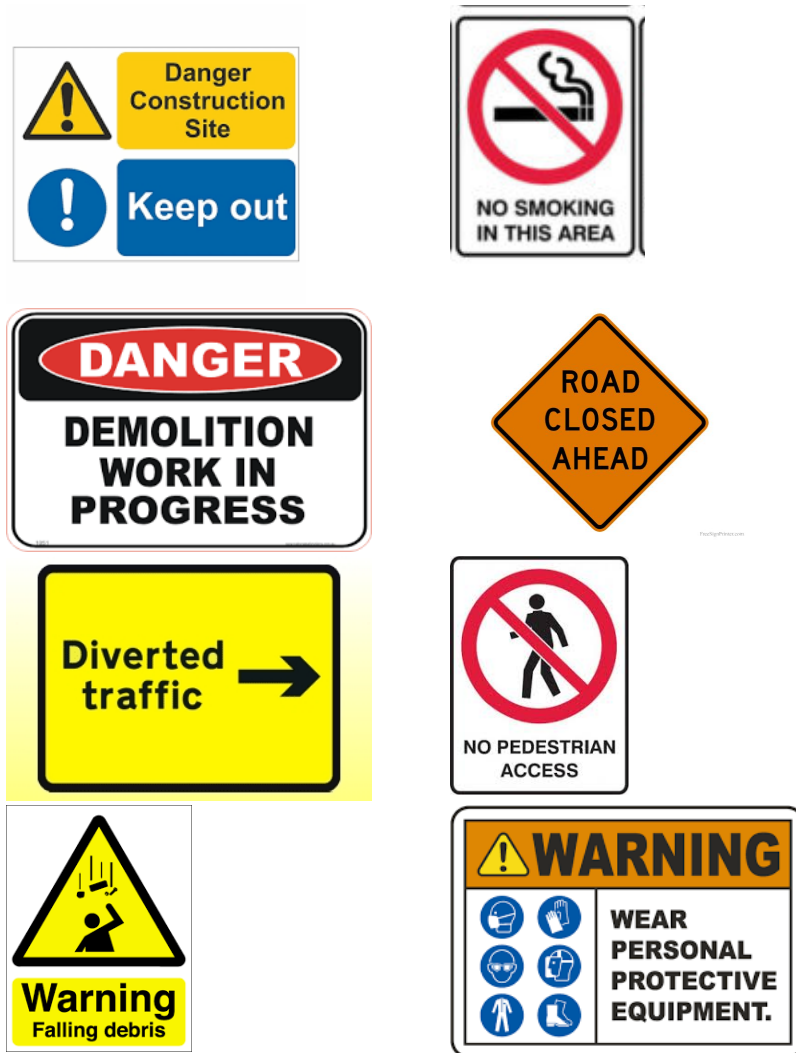
Figure 3-2: Signage for Demolition Site
