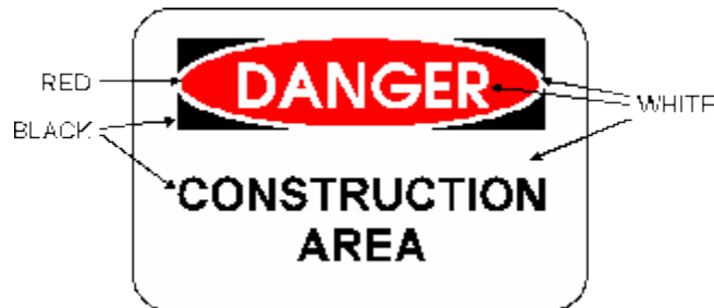
Figure 16. Example of the type of sign that should be visible on site when work is being performed.
